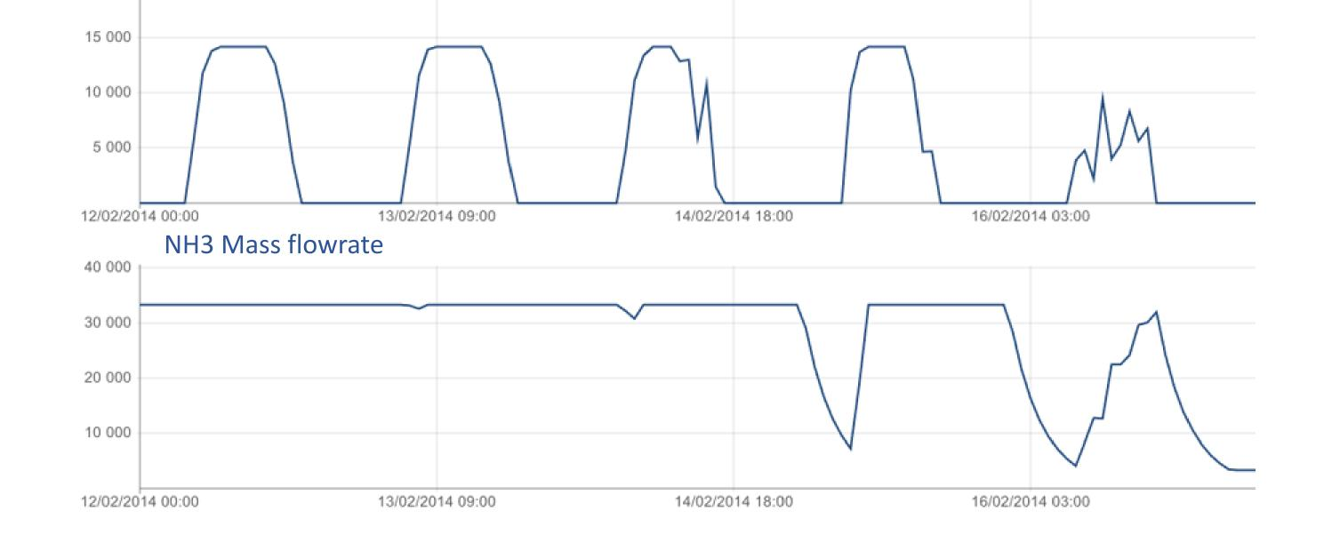
As an example, for a given solar farm capacity, it allows to define the best Ammonia plant capacity considering Hydrogen storage capacity variation (step 1), and ammonia plant production operation (fluctuating or constant) (step 2)
